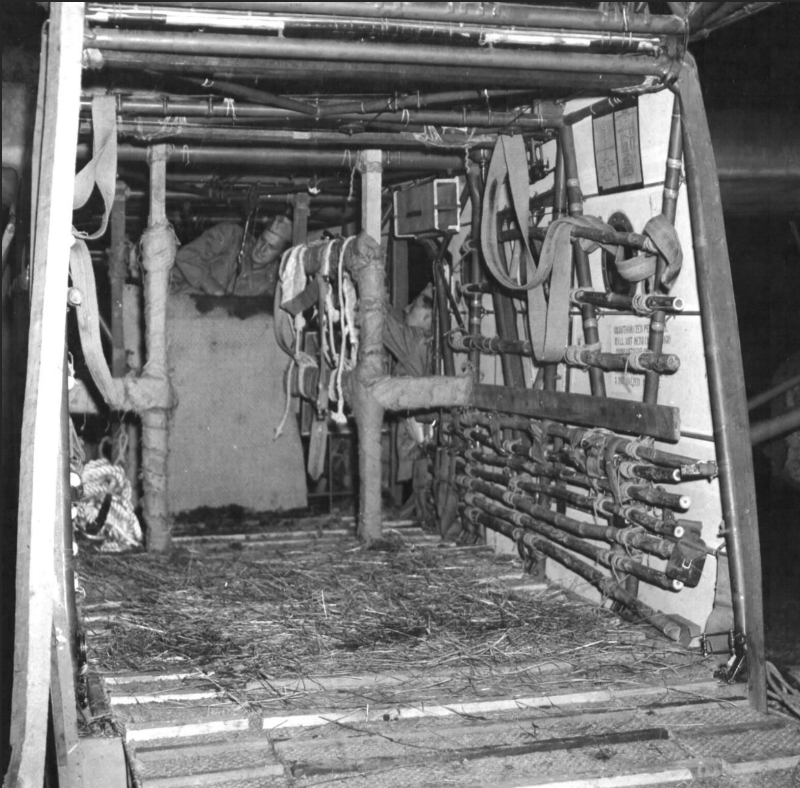
Padded glider (interior) with protective bamboo poles on side and straw matting on floor was used to transport mules in the maneuvers of the 1st Air Commando Force in India. —Photo curtesy of the U.S. National Archives
