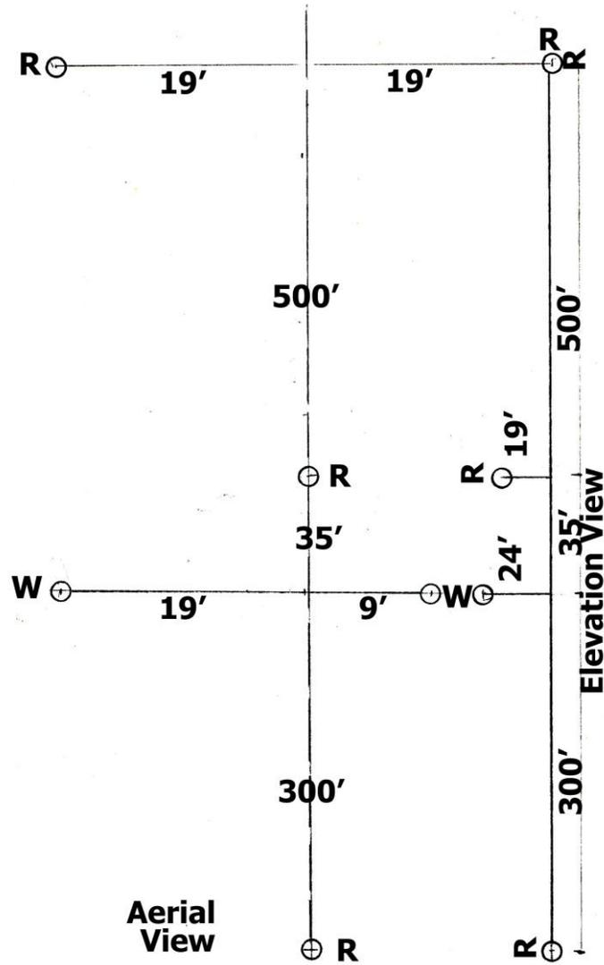
Aerial view depicting layout of poles and lights looking down to show the width and length of the light layout. The right edge (turn sideways) of depiction, marked Elevation, shows the height of the lights and poles relative to the ground.
